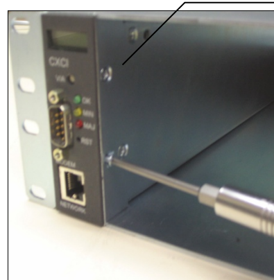
Figure 8—Showing CXCI module installation
