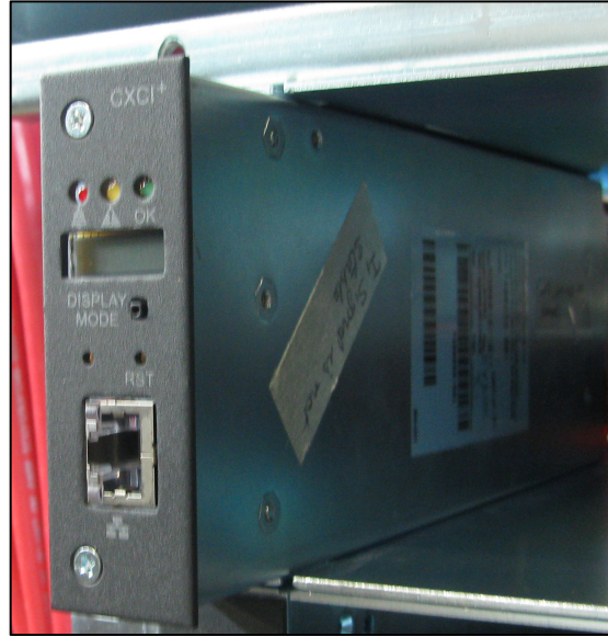
Figure 5—Showing CXCI+ controller module installation
