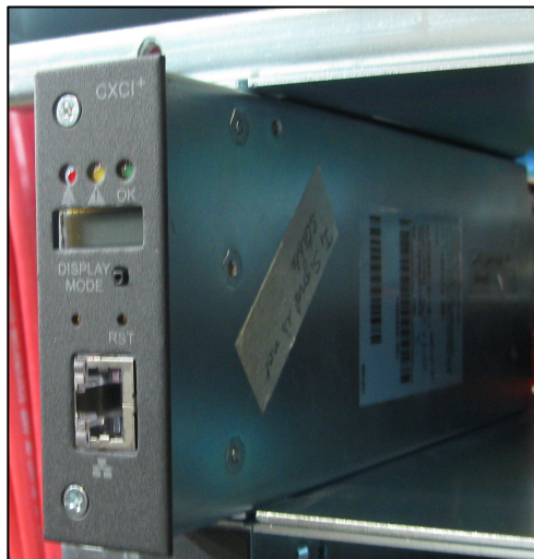
Figure 13—Cordex CXCI+ controller module
